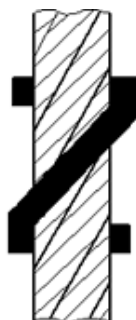
Right Hand Lang's Lay RHLL
