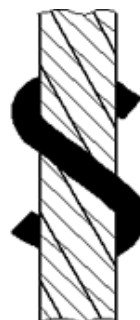
Left Hand Lang's Lay RHLL
